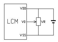
V<sub>DD~</sub>V<sub>0</sub>: LCD Driving voltage VR: 10k~20k
